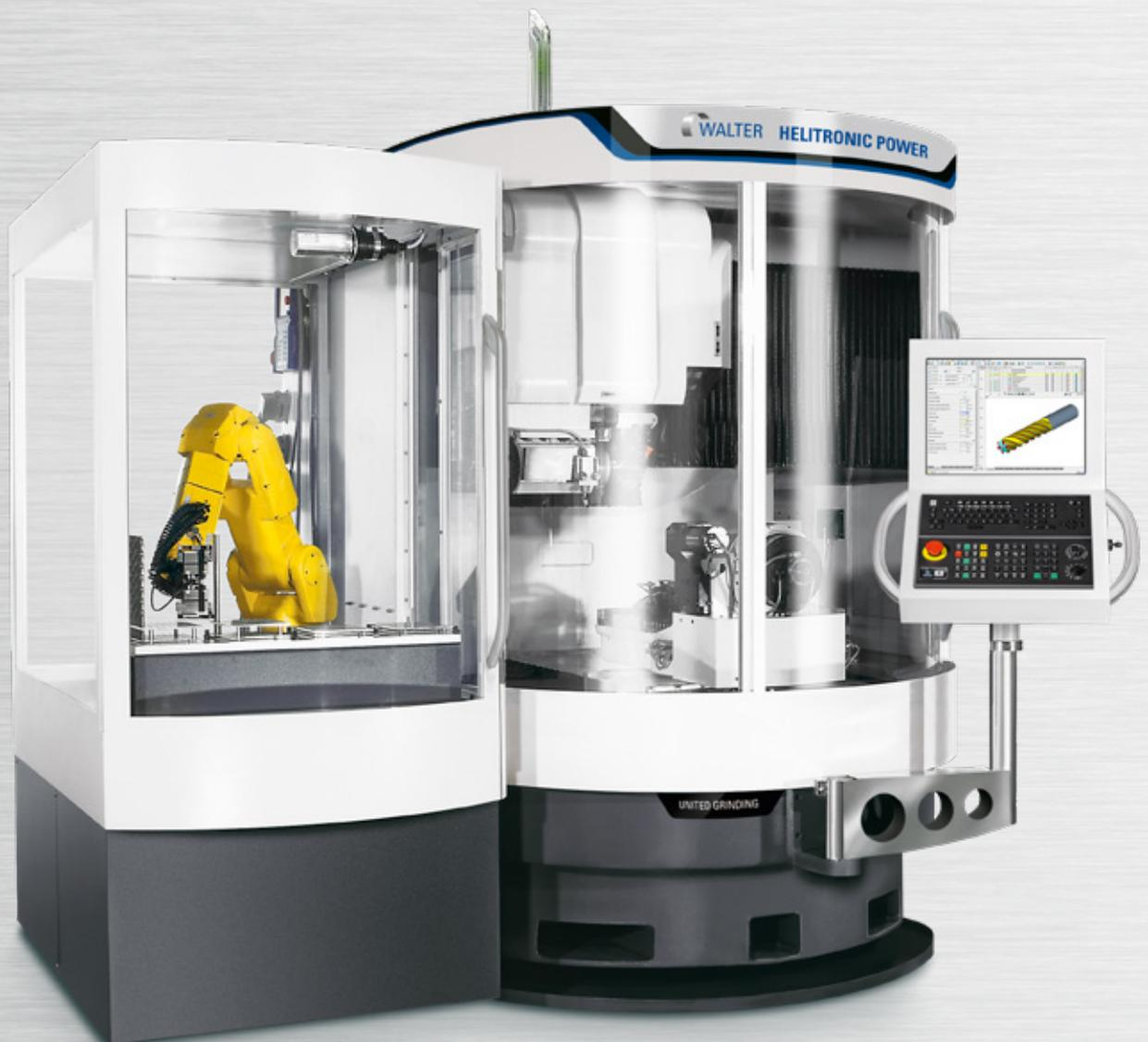
HELITRONIC POWER with Robot loader - the high level, high-performance version for minimally-manned multi-shift operation and mid-large volumes.
