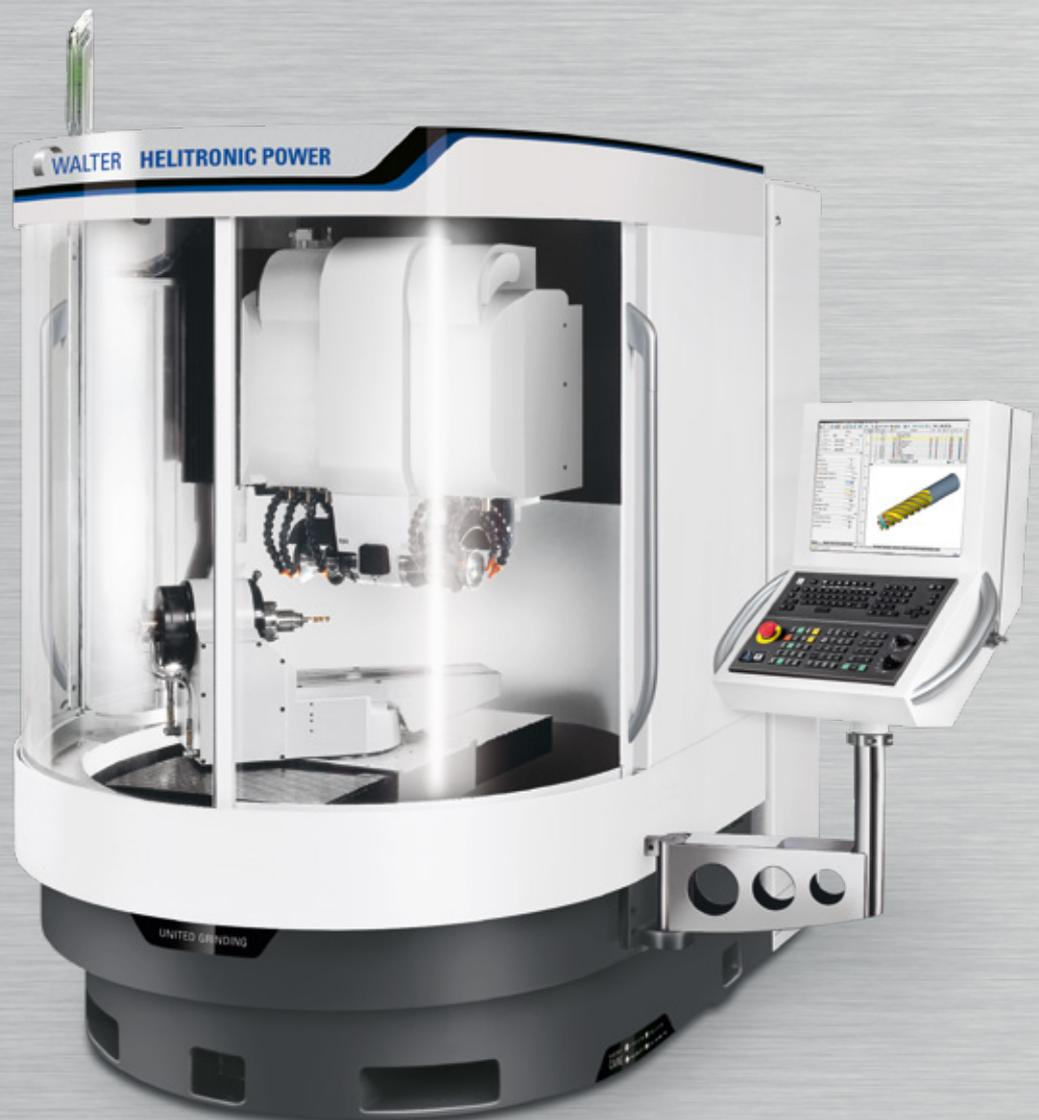
HELITRONIC POWER – the space-saving version with a belt-driven spindle and two ends.
