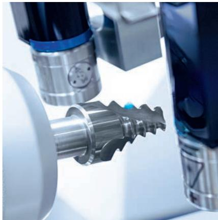
*The laser measures a milling cutter with a fir tree profile for the turbine industry*
