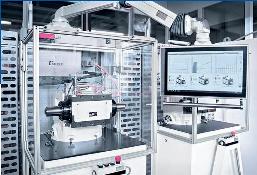
*The modernized spindle test benches are vibration-free, individually controllable, and feature precise sensor technology*
