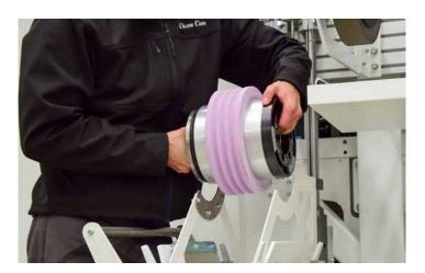
The loading device enables **easy and safe set-up** of grinding wheels during production. This further reduces the set-up times.
