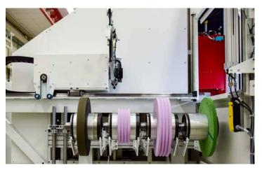
**High productivity** is achieved thanks to the possibility to prepare, for example, roughing and finishing wheels or conventional and CBN wheels in the changer, thus enabling both high stock removal rates and the precise finishing of surfaces in one operation.
